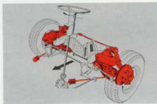
Independent front suspension and steering (LT 28/31/35).
